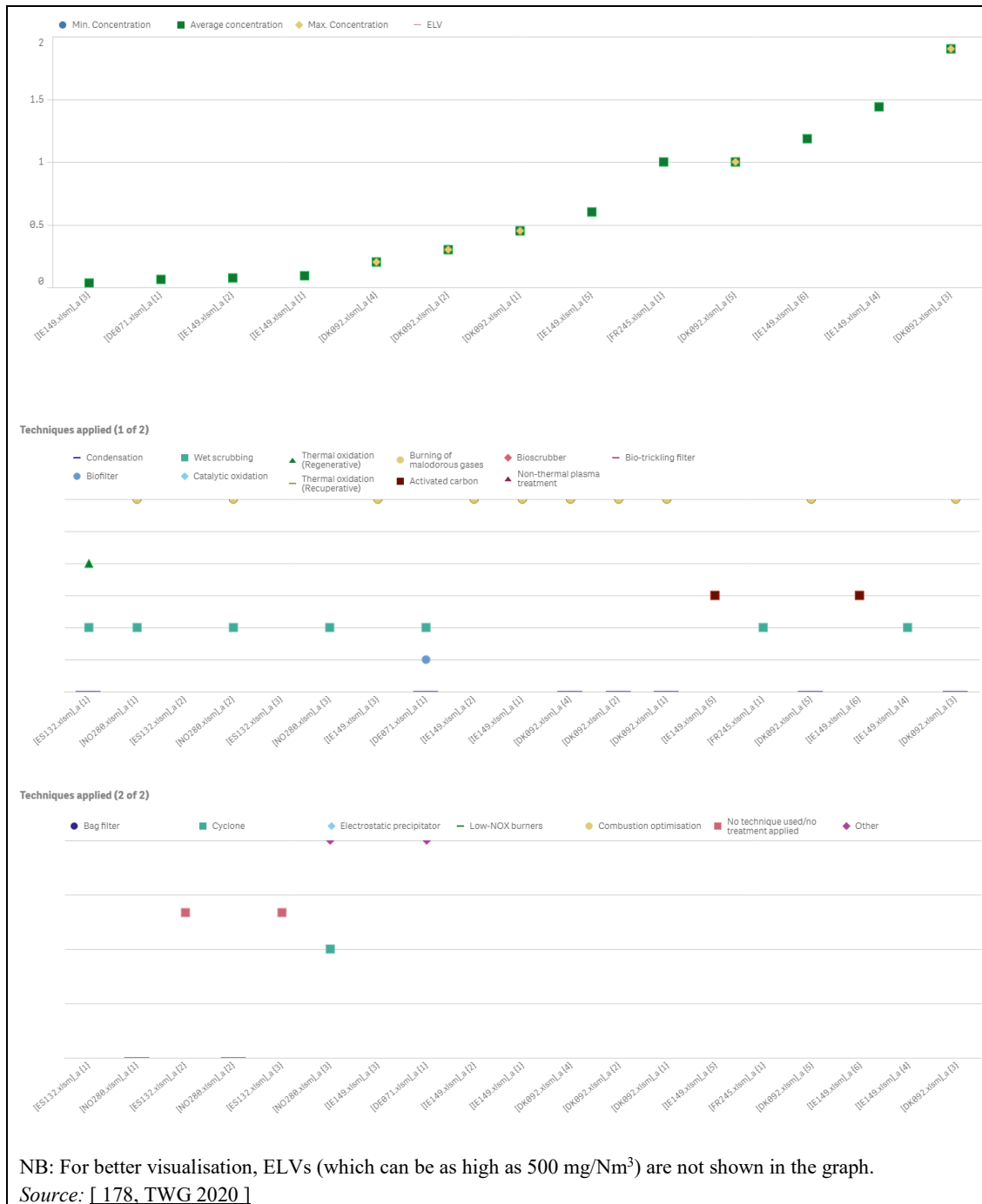
Figure 4.48: NH 3 emissions to air (mg/Nm 3 ) and abatement techniques from fishmeal and fish oil production
