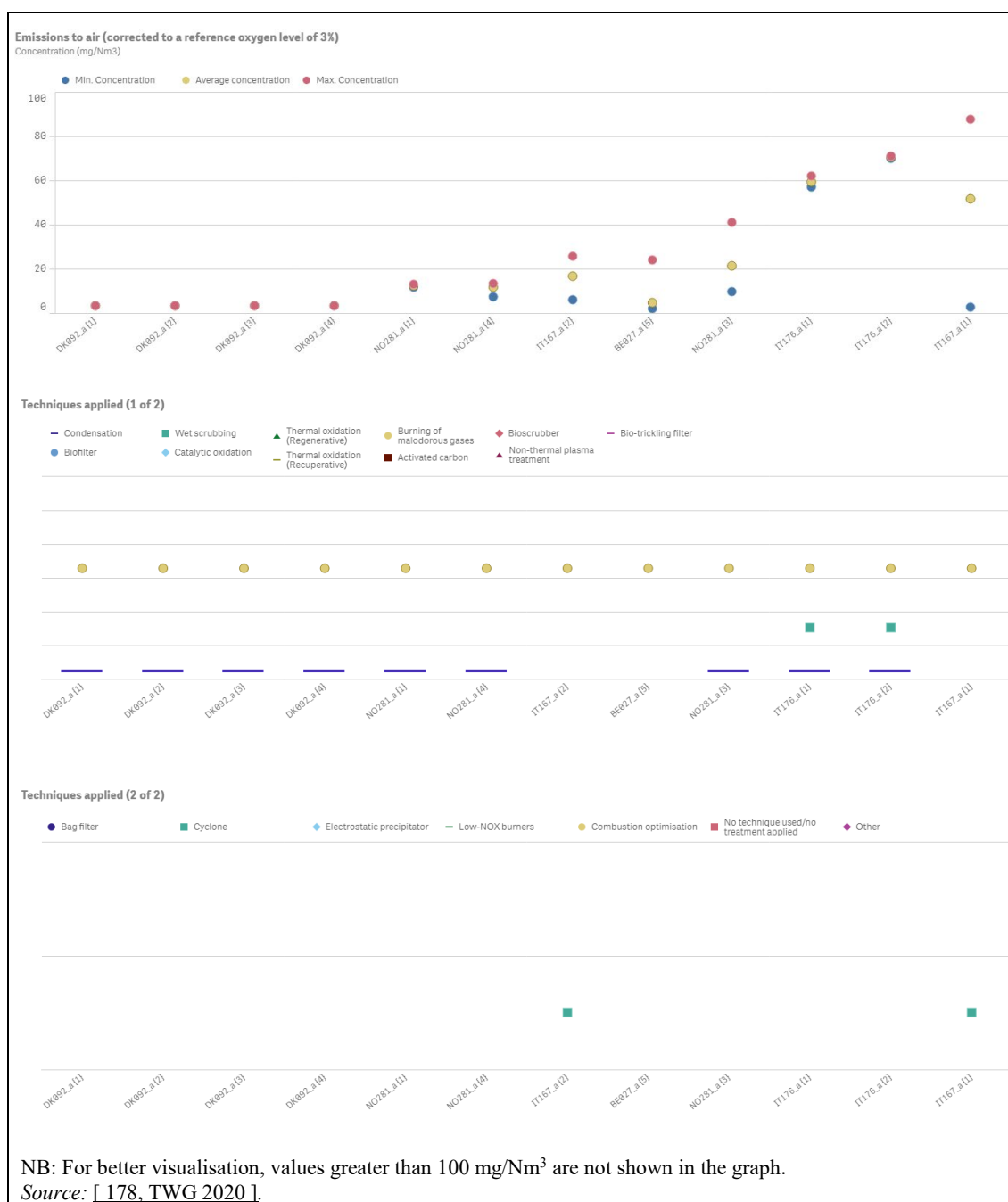
Figure 2.25: CO emissions to air (mg/Nm 3 ) from combustion in boilers of malodorous gases, including non-condensable gases, in SA installations (values corrected to 3 % O 2 )
