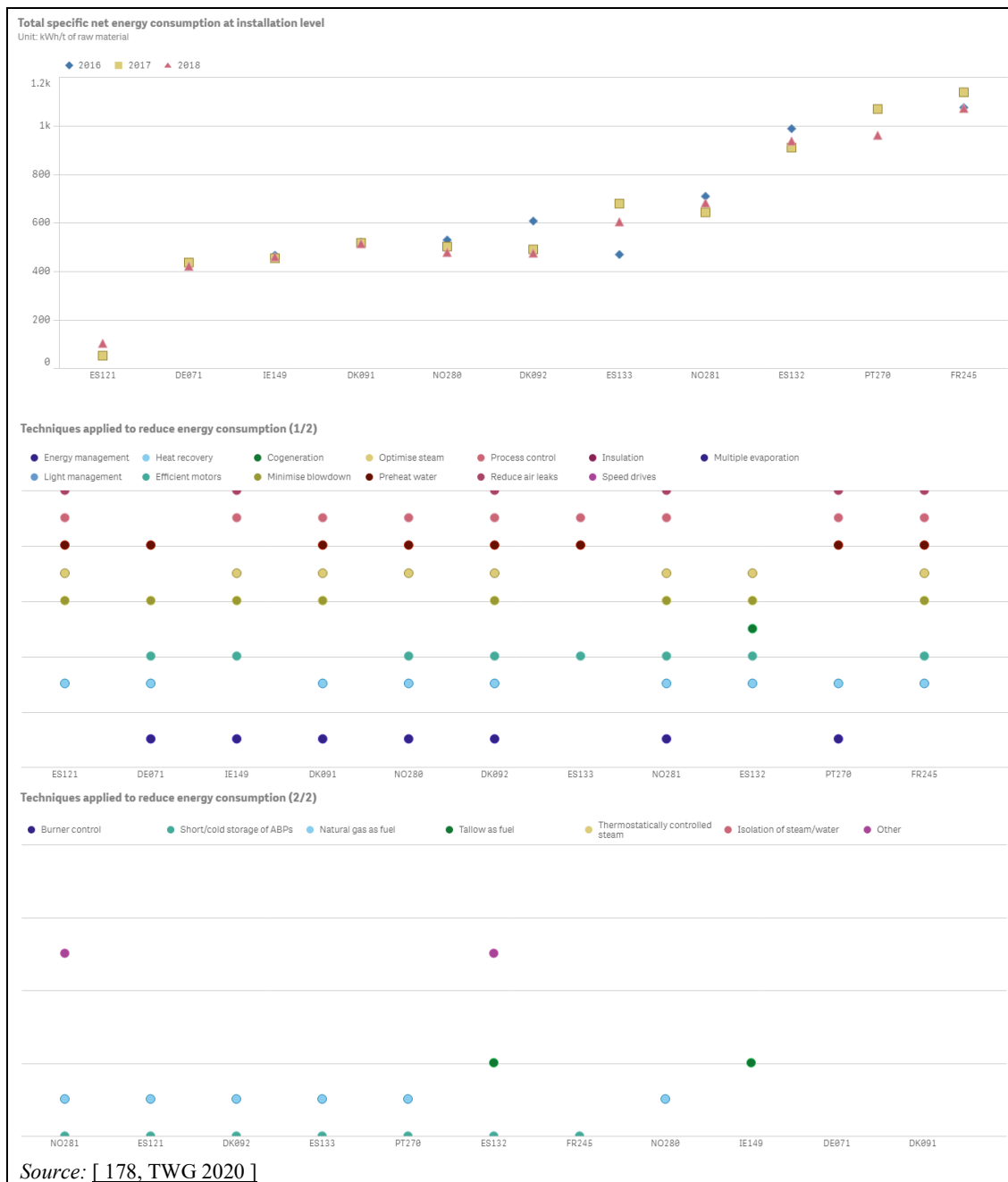
Figure 4.37: Specific net energy consumption (kWh/tonne of raw material) and applied techniques to reduce energy consumption in fishmeal and fish oil production (installation level)
